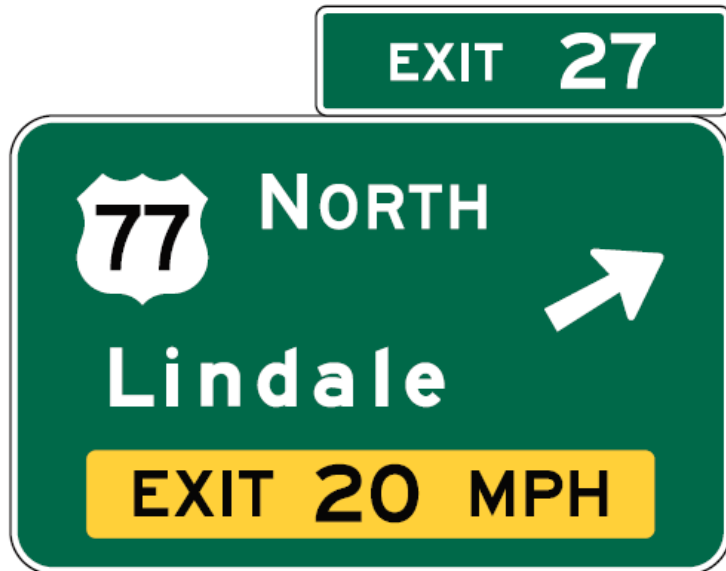
Exit Direction sign with E13-2 sign panel
