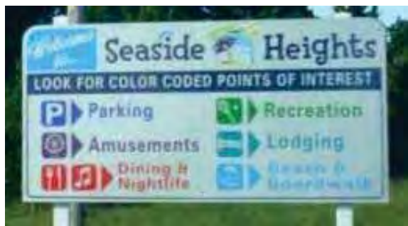
Incorrect use of boundary sign, excessive info
