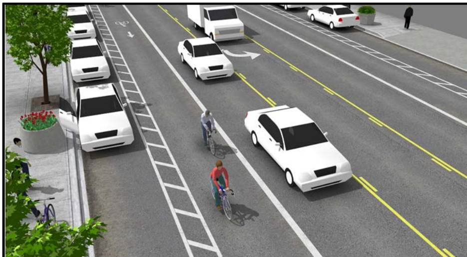
Figure 9 – 16 Buffered Bicycle Lane Adjacent to On-Street Parking
