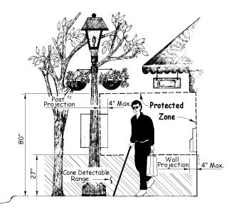
Intent is to eliminate objects that may protrude into the pedestrian path, reducing access and possibly causing injury
