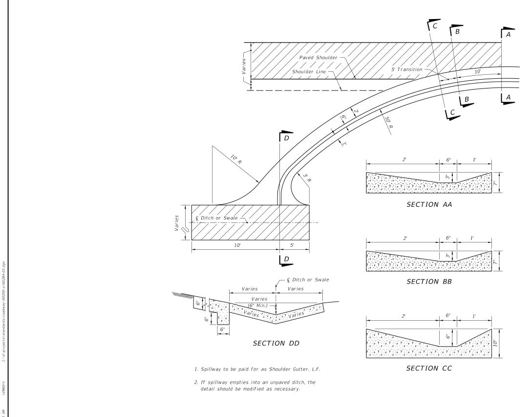
DETAIL OF CONCRETE SPILLWAY AT END OF SHOULDER GUTTER (TO BE USED WHERE INLETS, PIPES & ENDWALLS ARE IMPRACTICAL)
