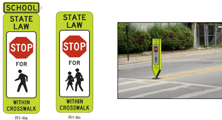
Figure 4: MUTCD R1-6 In-Street Pedestrian Signs
