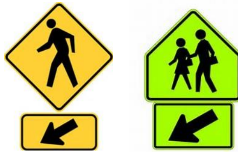
Figure 3: Example of MUTCD Crosswalk Signs with Arrow Plaque (Left: W11-2 Crosswalk; Right: S1-1 School Crossing)
