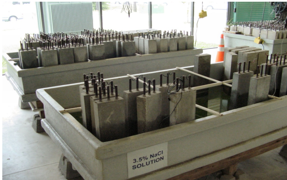
Figure 1c. Three-bar Tombstone Column Specimen Exposure
