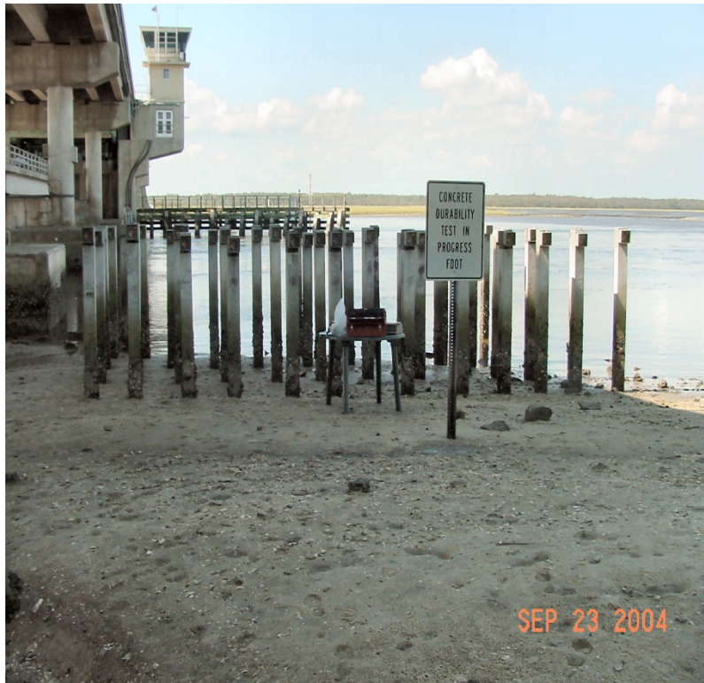
Figure 3b. Field Column Specimen Exposure
