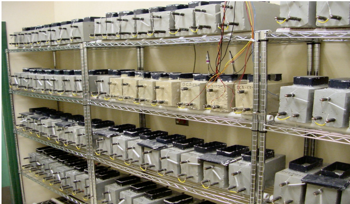
Figure 2c. G109 Specimen Exposure
