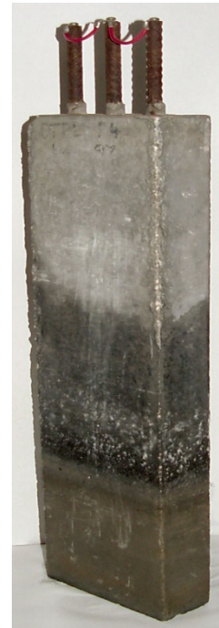
Figure 1b. Three-bar Tombstone Column Specimen
